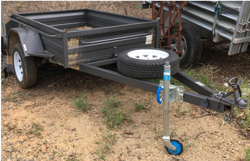
Figure 1: Existing powder coated trailer.
